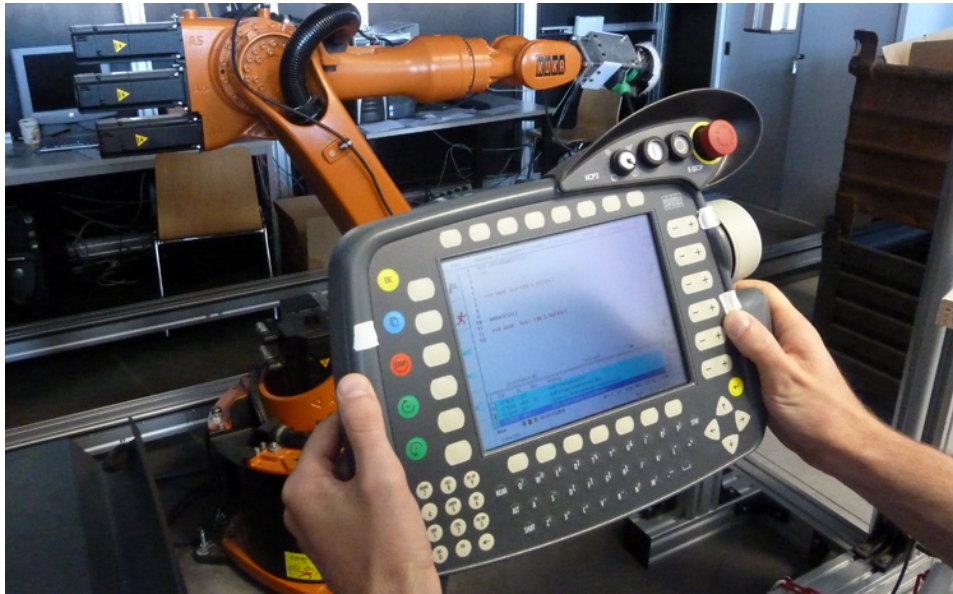
Figure 1.1: Teach pendants are used for programming and operating the robot within the workcell.
