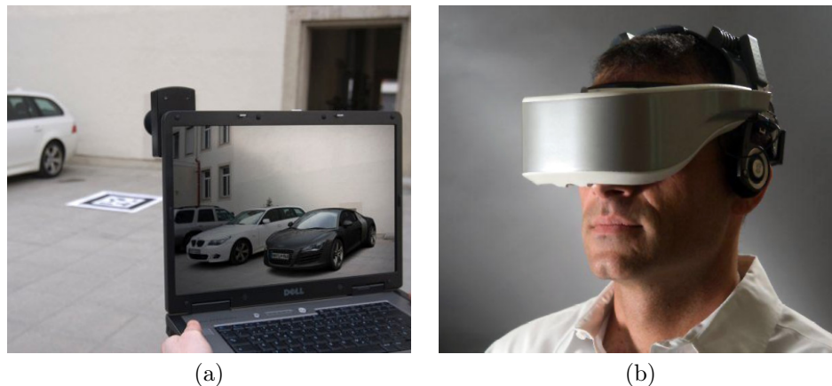
Figure 1.6: VST AR displays superimposed images on a screen (a). (Image courtesy of RTT AG.) The zSight is one of Sensics ' professional HMDs with high-resolution displays (b). (Image taken from http://sensics.com .)
