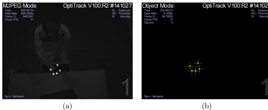
Figure 4.8: OptiTrack cameras can be operated in IR mode (a). The pre-processed, thresholded camera image already contains marker positions with subpixel accuracy (b).
