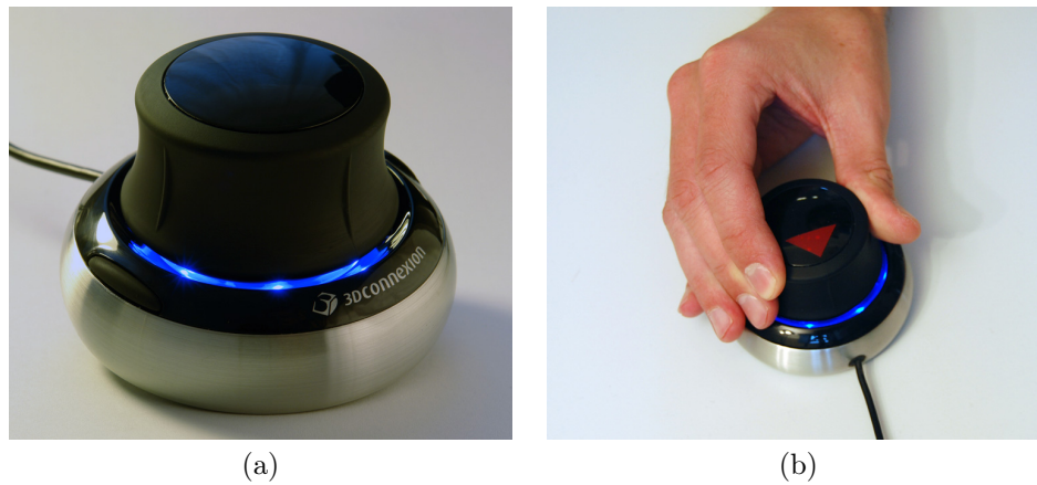
Figure 3.2: A 3Dconnexion SpaceNavigator 3D mouse was used for Teach Pendant (a). (Image taken from http://de.wikipedia.org .) It may be translated and rotated freely and thus provides 6 DOF (b).
