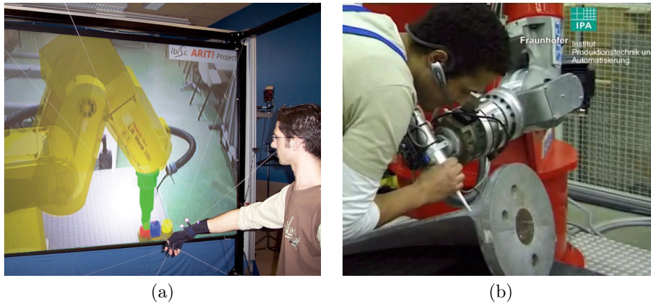
Figure 2.5: The data glove was one of several equivalent modalities, used to control the virtual robot arm (a). Force-torque sensors were used for the teaching of this gluing scenario (b).
